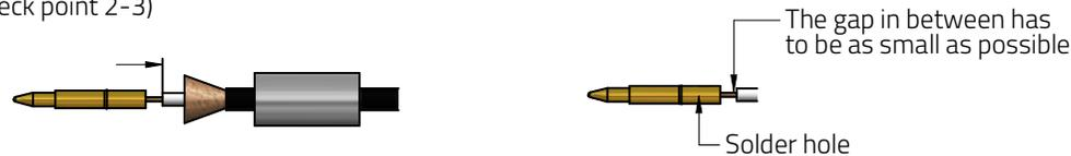
**Step 4.** Push cable with center contact into connector main body until perceptible point. Cover cable braid over connector neck carefully
