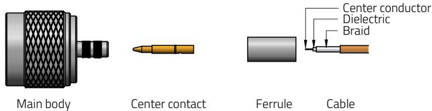
**Step 2.** Please slide ferrule onto cable and splay out cable braid
